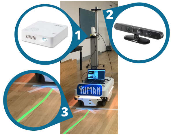
Fig. 2. MiR100 mobile robot used in our HRI experiments. We added an Asus Xtion Pro Live RGBD camera(1) and an Acer C202i projector(2). The projected image illustrates the robot’s navigation plan(3).
