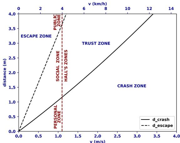
Fig. 5: Distances and zones predicted by the PTR model for different car speeds  $v$  at lower speeds.
