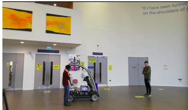
Fig. 6: OpenPodcar: open source hardware AV [15].
