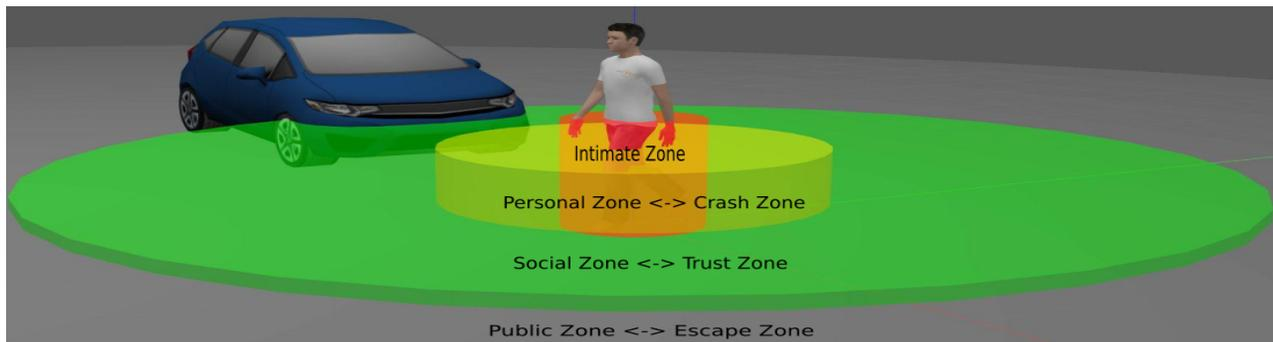
Fig. 4: Autonomous vehicle entering pedestrian’s social zone, which can also be viewed and quantified as a trust region.
